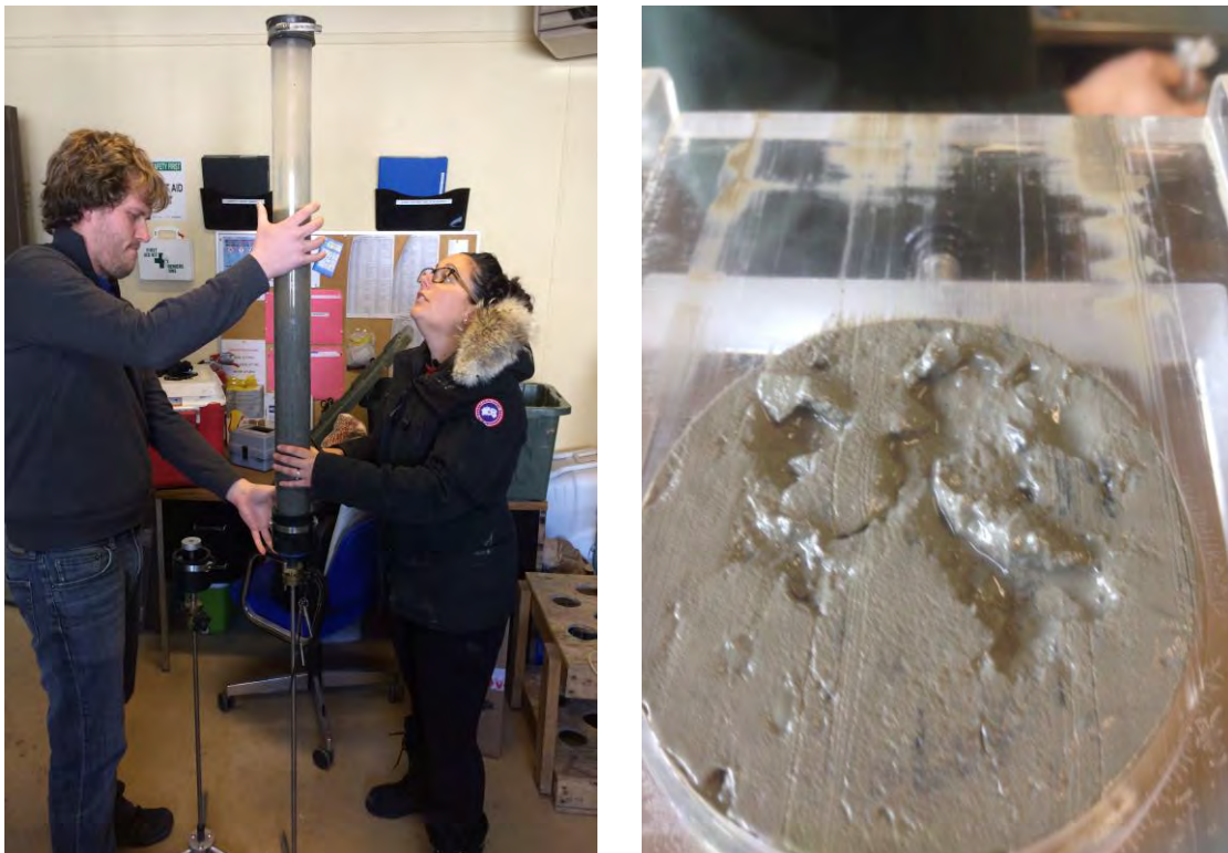
Figure 6: Back in the lab, the core was extruded (left) and subsampled (right).
